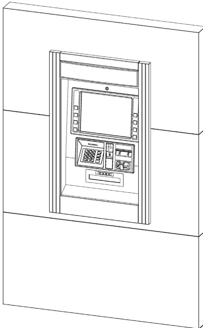
This document provides dimensions and specs for planning your GT5000 installation. The wall hole should be sized 35.7" (height) and 20.5" (width) as shown below.
