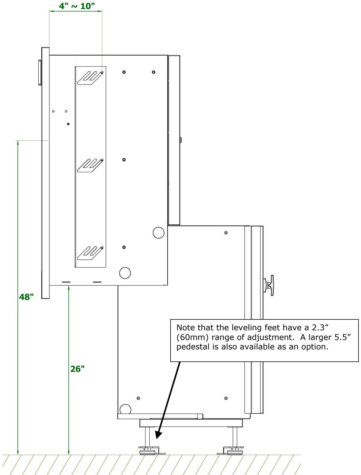
The following shows how to set the hole dimensions so that the machine will have the correct height for ADA compliance.
