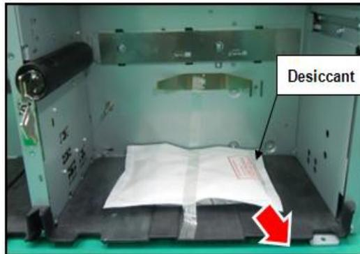
Removing the desiccant from the Bottom Section
