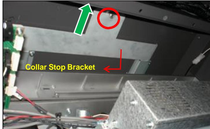
2. Lift the collar wing so that the pin at the back of the bezel fits into the hole.
