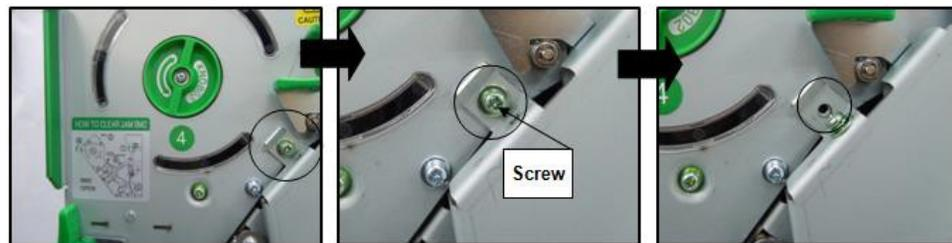
Removing the screw fixing the transport section of BM2
