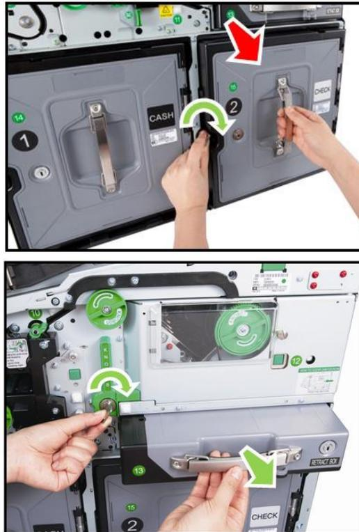
► Installing the PRT Cartridge Section
