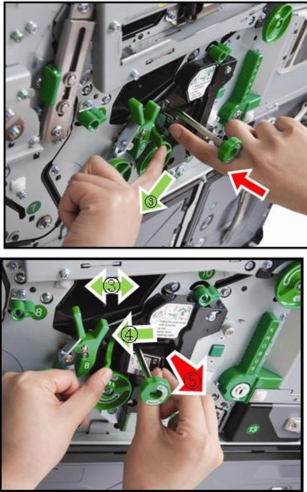
3. And then release the green grip, the ink cartridge is locked.
