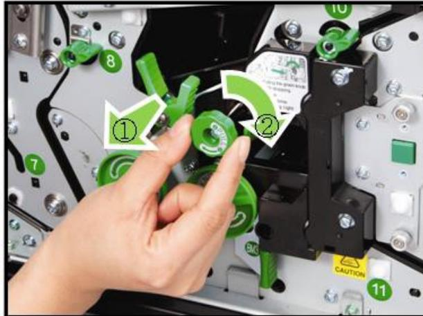
2. After opening the green grip (③), insert the ink cartridge in the cartridge adaptor (④).
