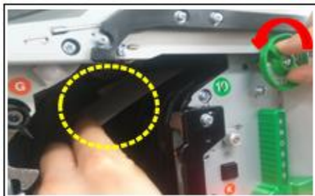
Remove bills and remained substance rotating KNOB05 three or four times.
