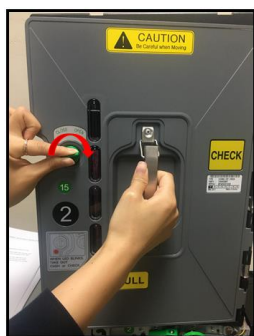
Open Cassette door using KNOB and handle
