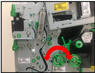
Remove bills and remained substance
