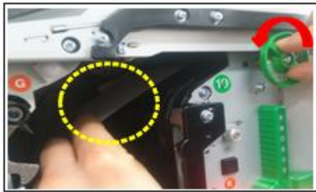
Remove bills and remained substance rotating KNOB three or four times
