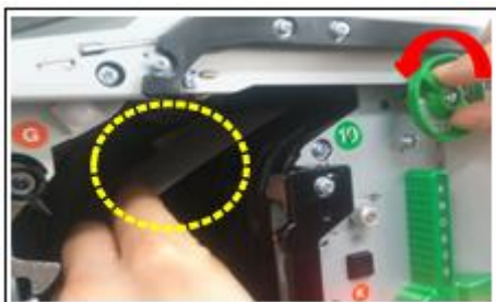
Remove bills and remained substance rotating KNOB05 three or four times
