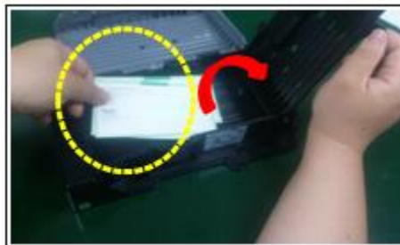
Once you open RT guide, Remove bills and remained substance
