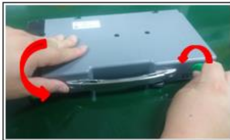
Once you close RT door, Lock RT door using KNOB
